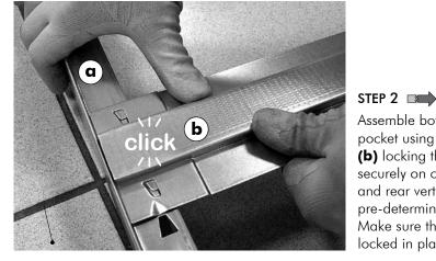
Assemble both sides of the pocket using the horizontals **(b)** locking them into position securely on central verticals (a) and rear verticals (c) at the pre-determined positions. Make sure they are firmly locked in place.
