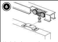
Hook the door onto the runners using the door brackets fixed to the top of the door. Insert the under door profile over the door guide and slide into the pocket. There is one adjustable stop already installed 70 mm from the rear of the track.
