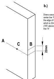
Draw a second center line "B" on the edge of the door which is 22mm (7/8") above center
