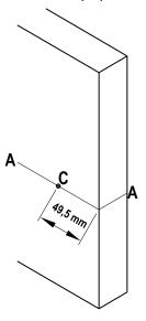
a.) Draw a level center line "A" on both sides of the door and on the edge of the door. The standard height for pocket door privacy kit is 1050mm (41 5/16") from finished floor. This centered line determines the position of the rose. Please mark the center of the rose with a distance of 49,5mm (1 15/16") from the edge of the door. Name
