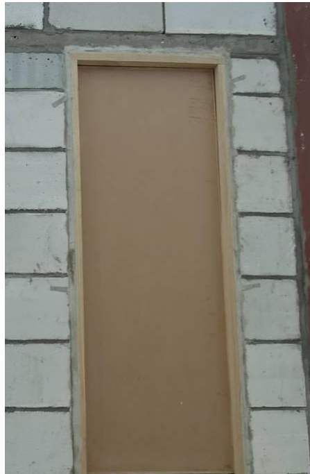
Fig. 1 - Exposed Side Prior to the Fire Test
