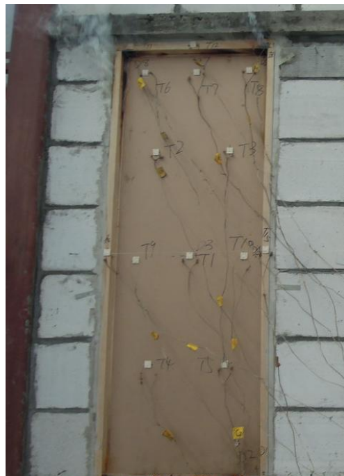
Fig. 4 – Unexposed Side after 30 Minutes
