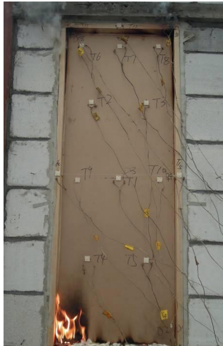
Fig. 5 – Unexposed Side after 40 Minutes
