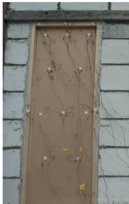
Fig. 2 - Unexposed Side Prior to the Fire Test
