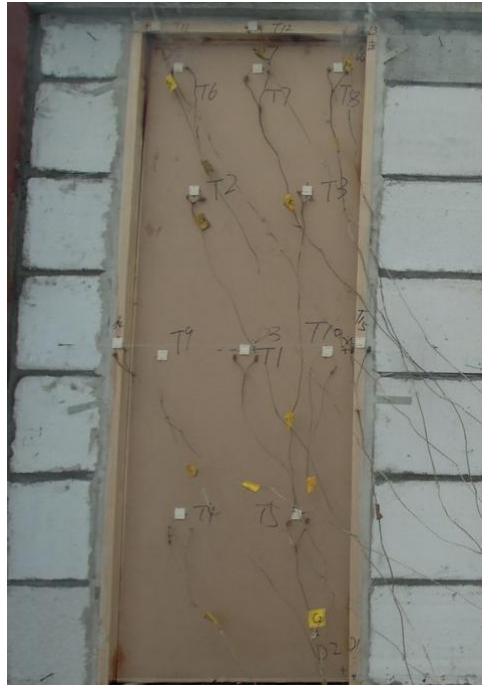
Fig. 3 – Unexposed Side after 7 Minutes
