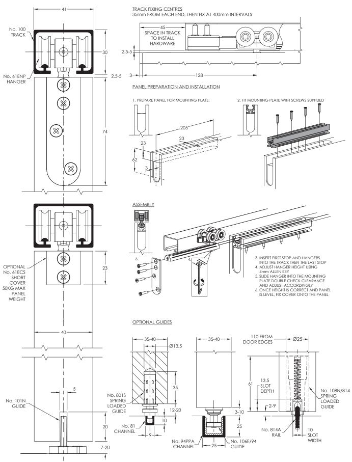
\* WHEN USING No. 100SCT SOFT CLOSE, 620 MIN PANEL WIDTH SINGLE SOFT CLOSE, 820 MIN PANEL WIDTH DOUBLE SOFT CLOSE
