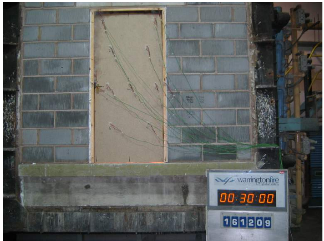
The unexposed face of the doorset after 30 minutes of testing
