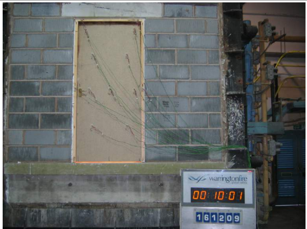
The unexposed face of the doorset after 10 minutes of testing
