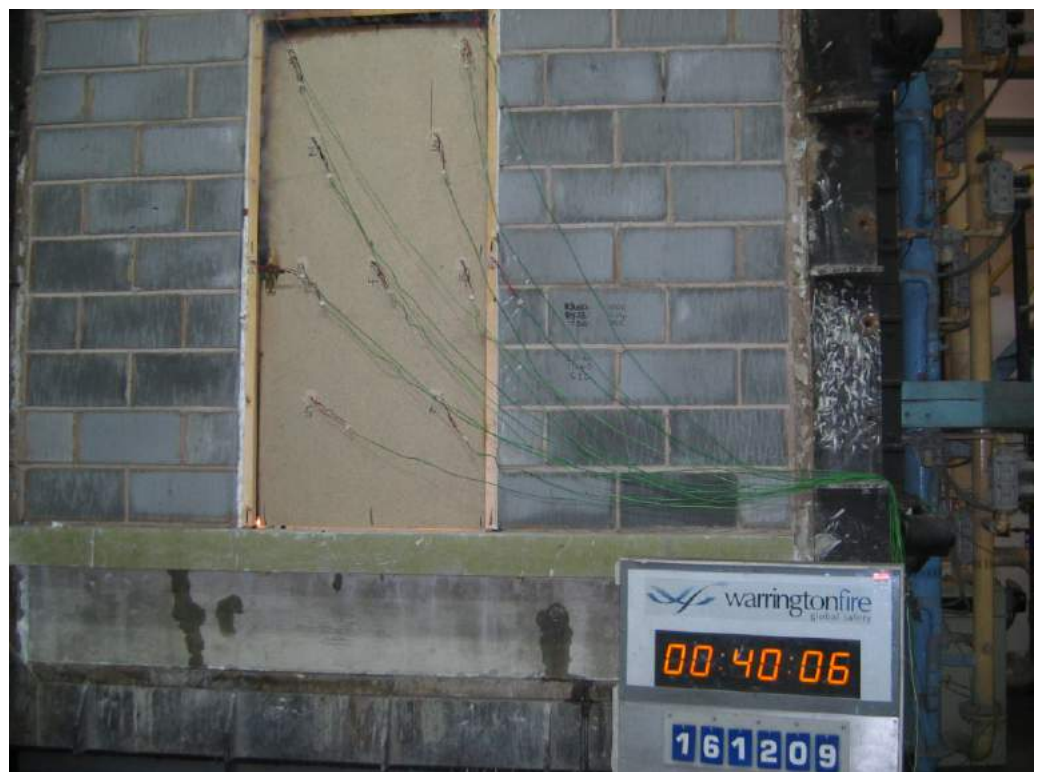
The unexposed face of the doorset after 40 minutes of testing
