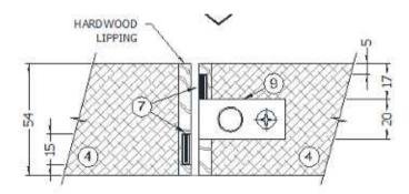
In addition the keep plate in the frame head shall be by-passed by the perimeter intumescent fire seals as follows for 60 minute applications only:
