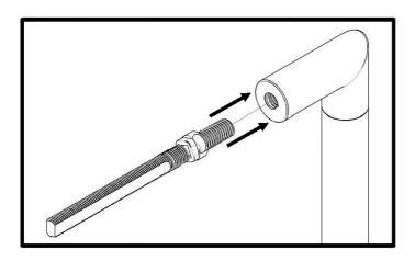
Securely fasten the short screw end of the two fixing bolts (1) onto both ends of the Tubular Handle fixing points.
