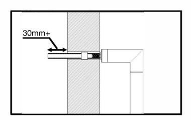
6. If the projection of the bolt from the face of the door is more than 30mm, it may be necessary to shorten the bolts.
