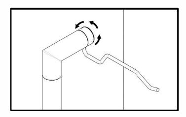
9. Continue to secure the pull handle to the door face by tightening the bush (5) progressively top and bottom until the pull handles are securely fastened to the door.
