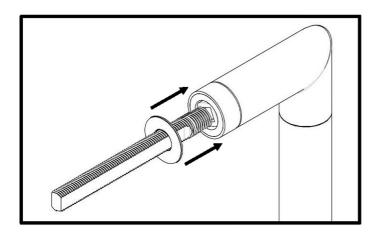
Slide one plastic washer (3) over each of the fixing bolts.
