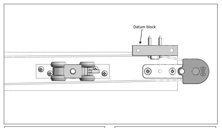
24. With doors in fully closed position, locate the clip stop by sliding the stop up to the lead door hangers and securing in position
