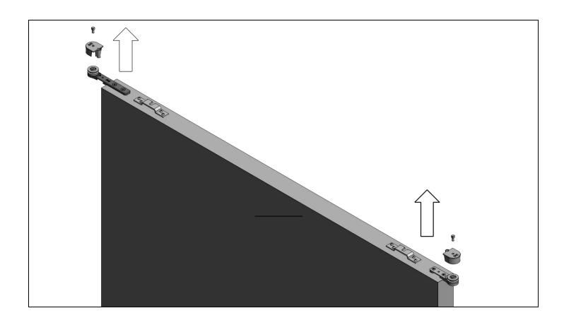
5. Loop belt around bearing wheels & cut belt to length
