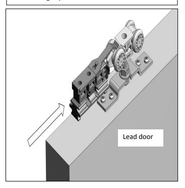
25. With all doors aligned in the open position, locate the clip stop by sliding the stop up to the lead door hangers and secure in position
