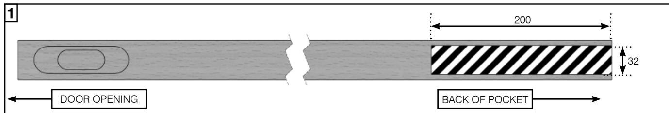
1. Cut the back of door mortise in the top of the door (200 x 32 x 30mm) and fix the bracket into this mortise. **(Screws not supplied)**
