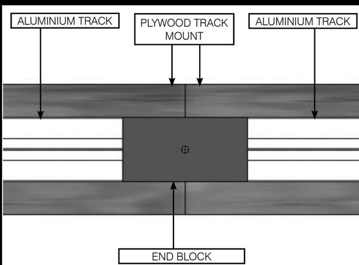
For **Double Door Kits**, cut the aluminium tracks to half the width of your horizontal studwork, minus 70mm.
