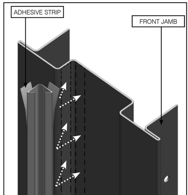
1. Cut the seals to the length of the front jamb. Peel back the adhesive strips and push in the two corners of the jamb.
