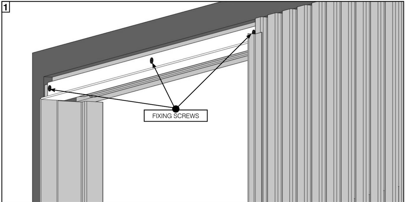
1. Cut the head jambs to fit the remaining door opening width. Screw into the track packers with '**Screw Set A**'.
