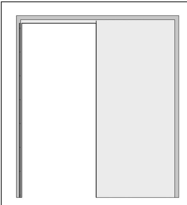
1. Clad the kit in 12.5mm of plasterboard. Ensure it butts up level and tight against all jambs.
