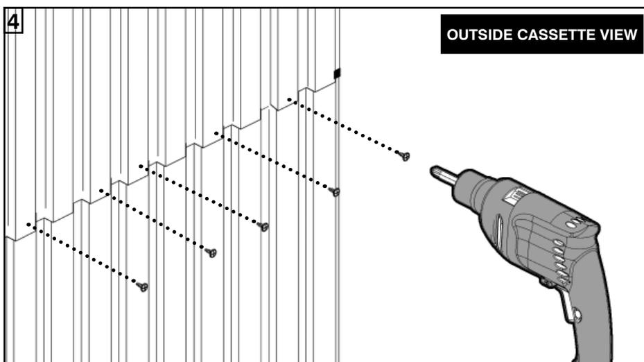
4. Pilot and screw through from outside to join panels together in five locations using 'Screw Set A'
