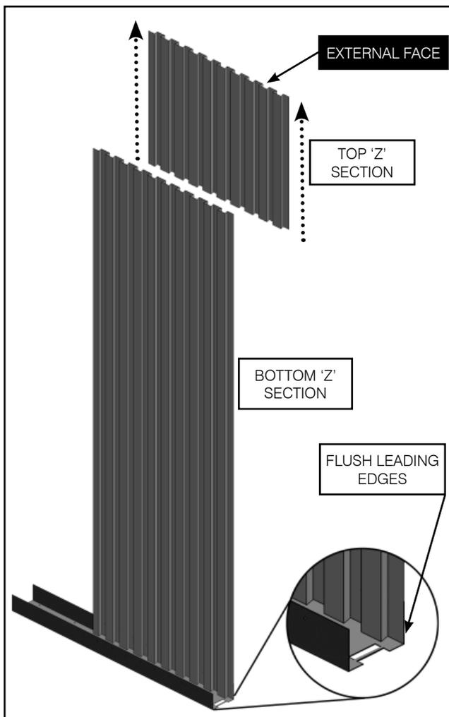
1. Extend the 'Z' Panels to desired height (inside surface of sole plate to underside of top studwork).
