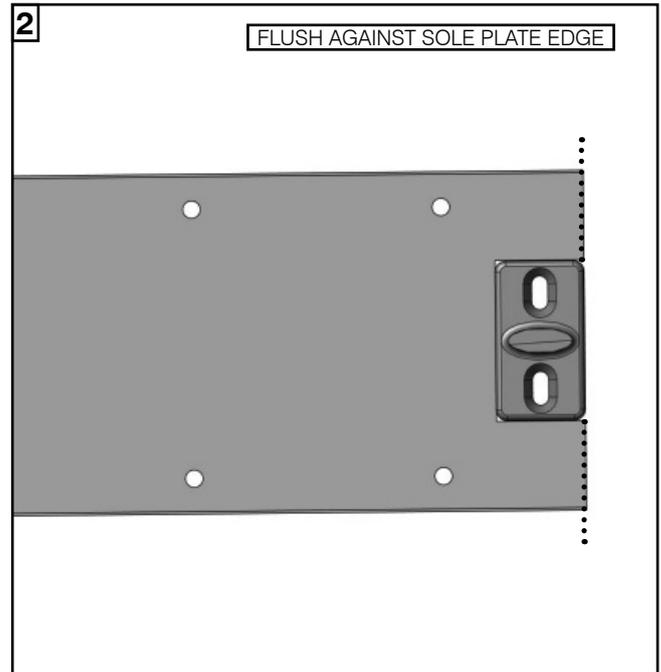
1. Fix the metal floor guide into the sole plate by inserting it into the pre-cut area.
