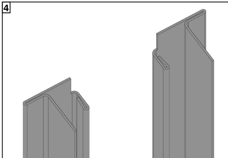
5. Insert the top of the jamb into the slot provided in the track packer.
