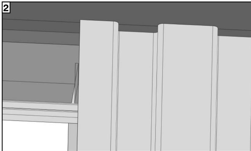
3. To secure the track packers, first pilot and countersink a series of holes in their length, approximately 300mm apart. Screw through into the plywood track mount using **'Screw Set E'**.
