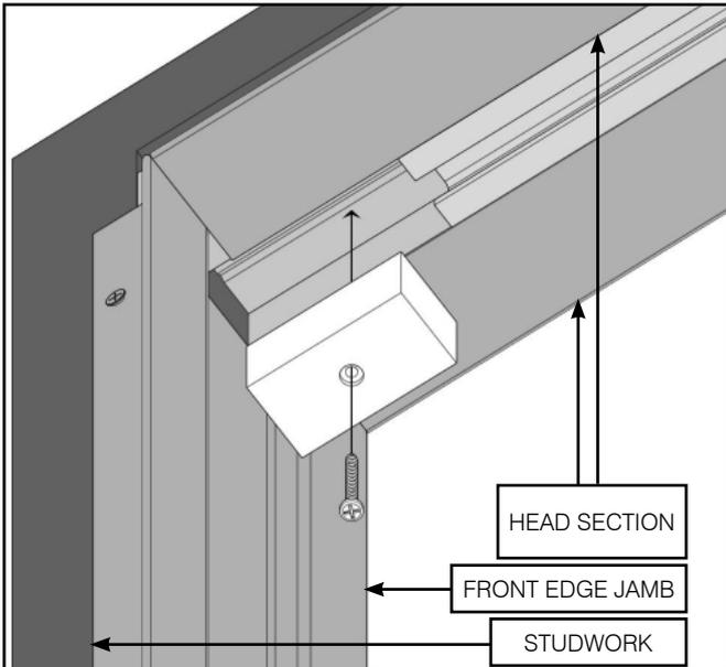
1. Pilot drill and counterbore a hole in the wooden end block using a 2mm drill bit. Drill the hole in the centre of the block.
