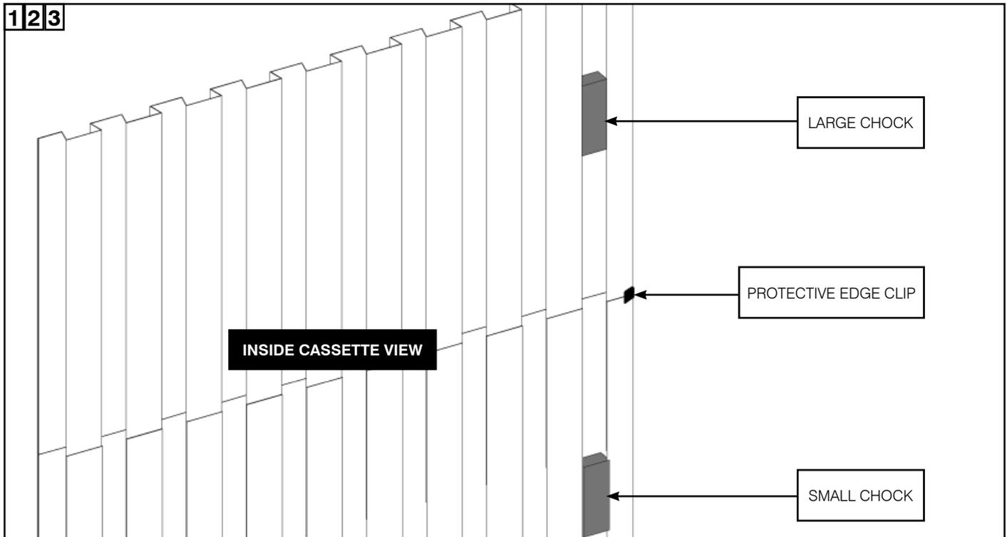
1. At the back of the pocket, place the protective edge clip onto the 'Z' section, covering where the panels join.
