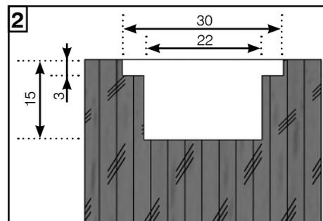
2. Cut the front mortise in the top of the door in two depth stages as pictured. Fix the flush bracket front plate over the mortise using supplied screws. Ensure the larger hole in the front plate is towards the front of the door.
