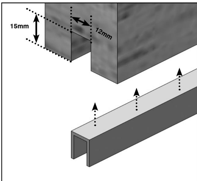
1. Cut a groove in the bottom face of the door to suit the plastic channel which the floor guide runs in.
