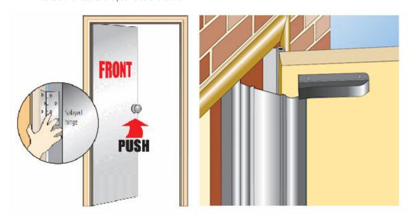
• 40903.1 is fitted on the rear pull side (knuckle side) of the door.
