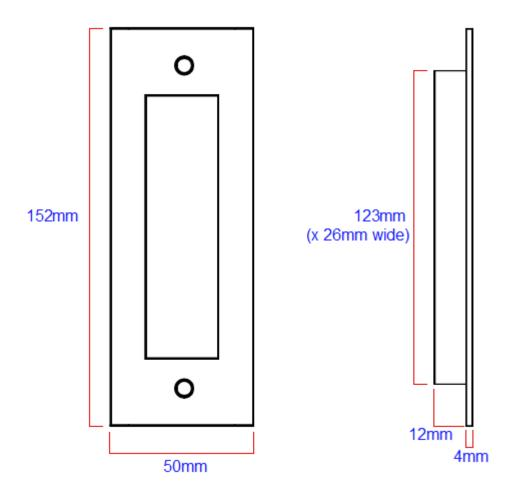
Item CodeHeightWidthRecess DepthRecess HeightRecess WidthBackplate Thickness40924.1152mm50mm12mm123mm26mm4mm
