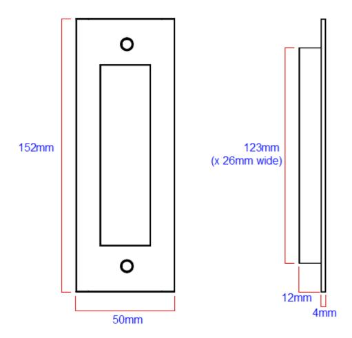
Item CodeHeightWidthRecess DepthRecess HeightRecess WidthBackplate Thickness40928.1152mm50mm12mm123mm26mm4mm
