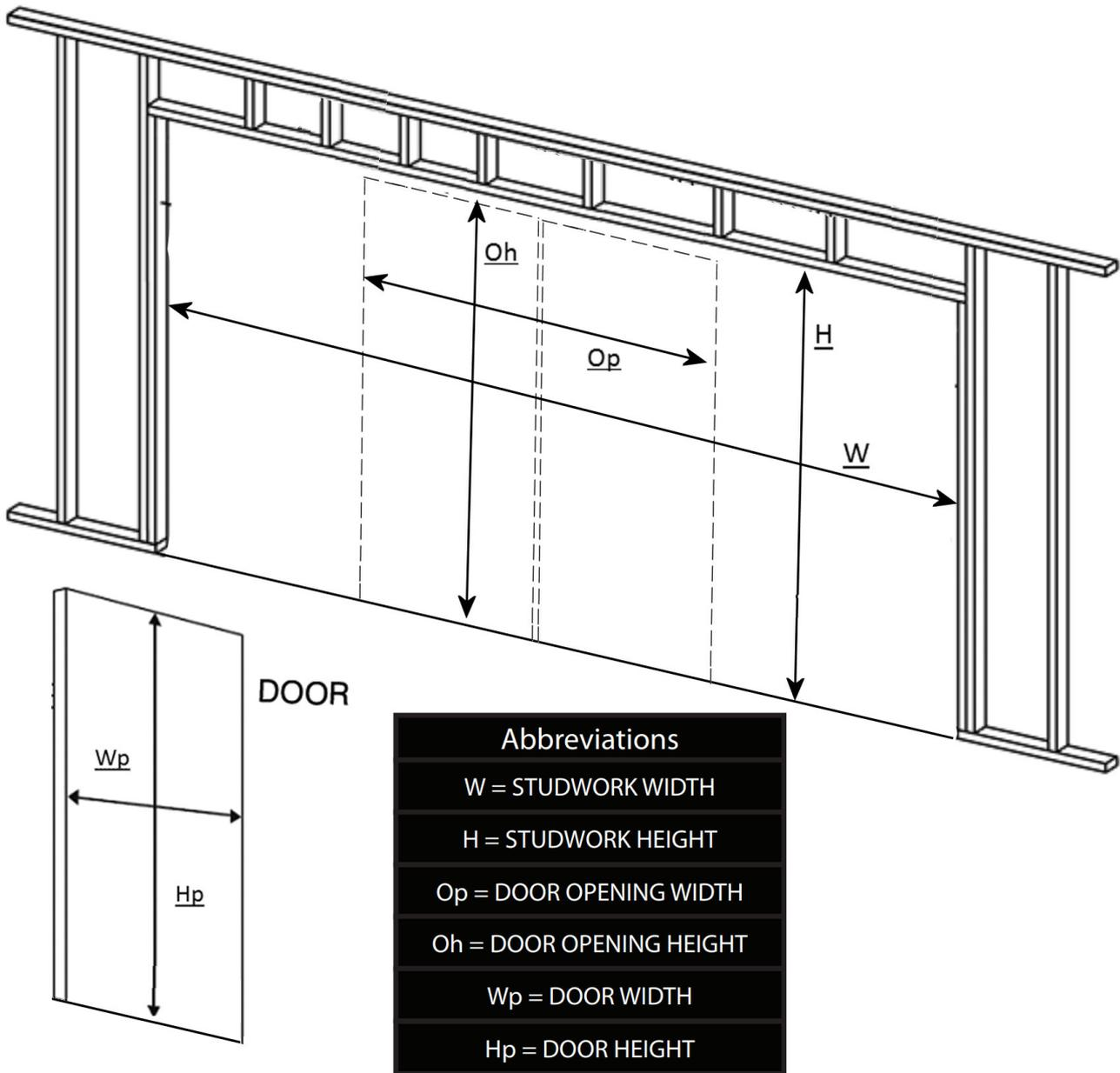
**To calculate studwork width and height from known door dimensions:**
