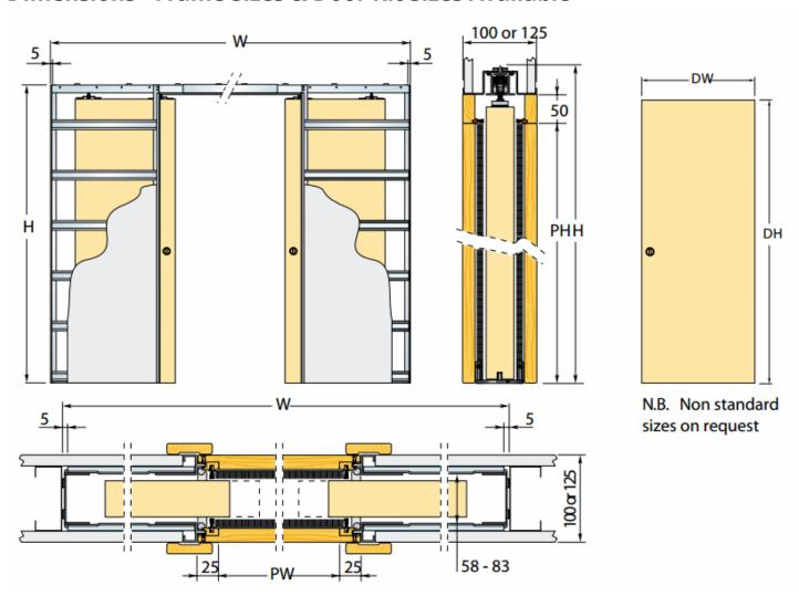
Item Code | Door Size - Each Door (DW x DH) | Max Passage Size (PW x PH) | Overall Frame Size (W x H) | Finished Wall Thickness
