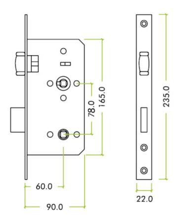
Item Code Lock Case Depth (A)Backset To Keyhole (B)Spindle To Spindle centers (C)
