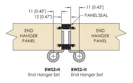
• End panel to swing configuration with non-non mortice hinges and square (plain) edge doors.
