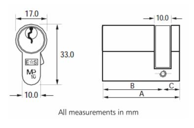
Item CodeOverall Length (A)External Side (B)Internal Side (C)CYH71146BK46mm36mm10mm
