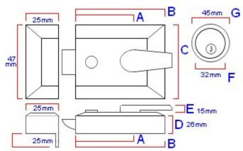
Available in two sizes - Backset size (Distance from edge of door to centre of the cylinder)
