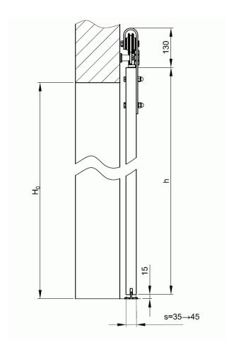
• Door height (h) is calculated as follows Ho (Opening Height) + 73mm
