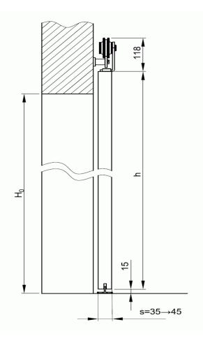
• Door height (h) is calculated as follows Ho (Opening Height) + 25mm
