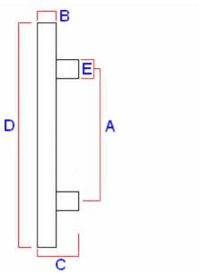
Item Bolt centers (A)Diameter (B)Projection (C)Overall Length (D)Post Diameter (E)
