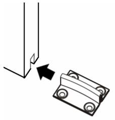
• "L" shape door guide is installed at the bottom (near the leading edge) of the 1st door panel and guides the 2nd door panel.
