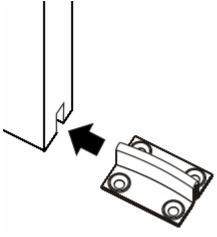
• "L" shape door guide is installed at the bottom (near the leading edge) of the 1st door panel and guides the 2nd door panel.
