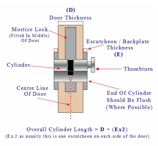
Always check the mortice lock is fitted in the middle of the door if not an offset cylinder is required
