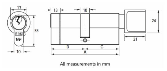
Equal cylinders for use with timber doors or doors with a mortice lock fitted in the middle of the door.
