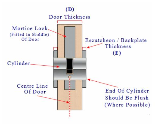
Overall Cylinder Length = D + (Ex2)(Ex 2 as usually this is one escutcheon on each side of the door)
