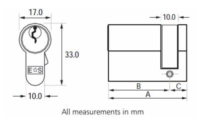
Item CodeOverall Length (A)External Side (B)Internal Side (C)43962.145mm35mm10mm
