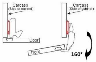
• Suitable only for doors that overlay the cabinet carcass - (see below diagram)
