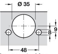
**Drilling pattern for screw fixing**
