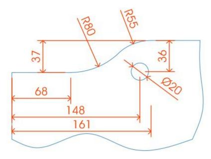
• Bottom patch / closer cut-out required in glass door (see below diagram):
