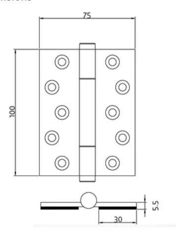
Height (H)100mmWidth (W)75mmLeaf Width30mmThickness5.5mm (Including Intumescent Backing)
