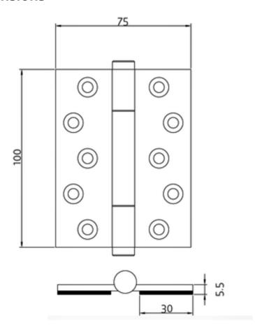
Height (H)100mmWidth (W)75mmLeaf Width30mmThickness5.5mm (Including Intumescent Backing)
