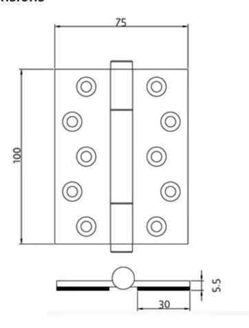
Height (H) Width (W) 75mm **Leaf Width** 30mm **Thickness** 5.5mm (Including Intumescent Backing)
