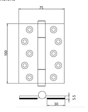
Height (H) Width (W) 75mm **Leaf Width** 30mm **Thickness** 5.5mm (Including Intumescent Backing)
