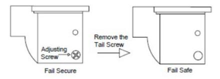
• This electric release is supplied as fail secure operation but can easily be changed to fail safe by the simple removal of a screw.
