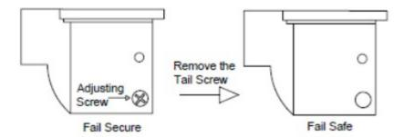
• This electric release is supplied as fail secure operation but can easily be changed to fail safe by the simple removal of a screw.
