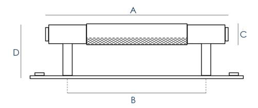
Item Code Overall Length (A)Fixing Centres (B)Bar Diameter (C)Projection (D)Backplate Length (E)Backplate Width (F)
