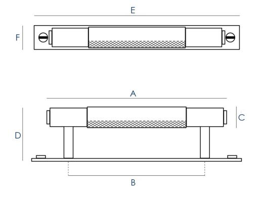
Item Code Overall Length (A)Fixing Centres (B)Bar Diameter (C)Projection (D)Backplate Length (E)Backplate Width (F)
