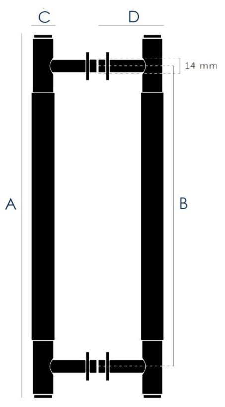
Item Code Overall Length (A)Fixing Centres (B)Bar Diameter (C)Projection (D)To Suit Door Thickness
