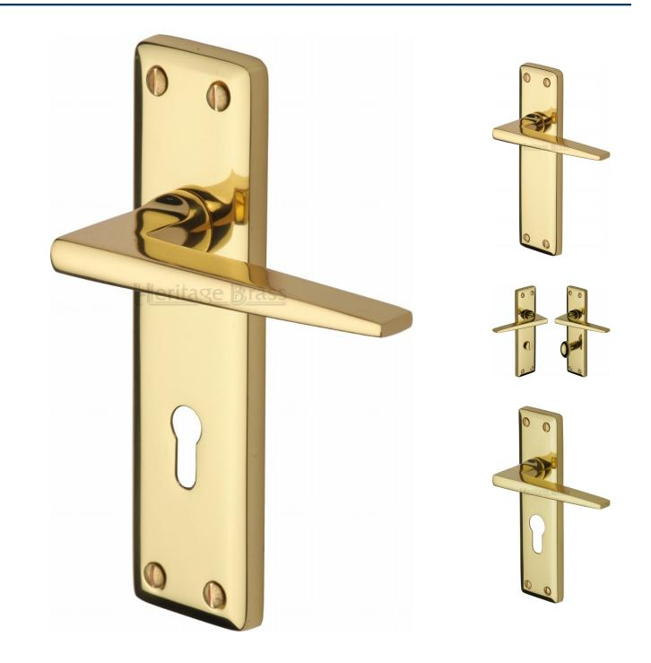
Available in various plate designs including latch set for non locking doors, lock set for key locking doors, bathroom set that locks via a thumbturn and can be released in an emergency via a coin release on the outside handle, and a euro profile set for use with euro profile cylinders.
