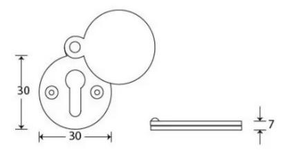
Overall Size: 30mm DiameterOverall Thickness: 7mm
