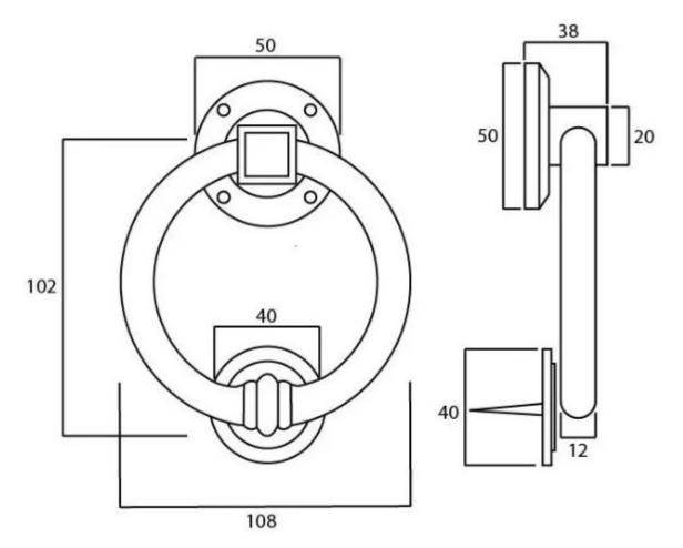
Ring Width: 108mmRing Length: 108mmFixing Plate: 50mm diamterProjection: 38mm
