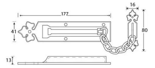
Fixing Plate: 177mm x 41mm
