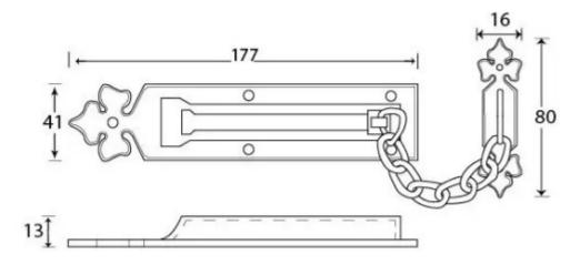
Fixing Plate: 177mm x 41mmChain Plate: 80mm x 16mm
