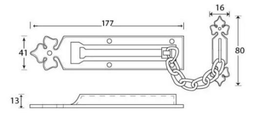
Fixing Plate: 177mm x 41mmChain Plate: 80mm x 16mmChain Length: 154mm
