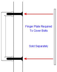
Above diagram shows how a bolt through pull handle is fitted to a wooden door  $% \left\{ 1\right\} =\left\{ 1$
