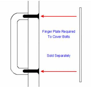
Above diagram shows how a bolt through pull handle is fitted to a wooden door
