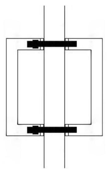
Above diagram shows how a bolt through pull handle is fitted to a wooden door  $% \left\{ \left( 1\right) \right\} =\left\{ \left$
