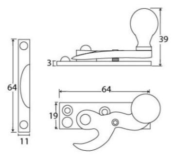
• Fixing plate: 64mm x 19mm
