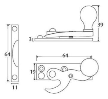
• Fixing plate: 64mm x 19mm
