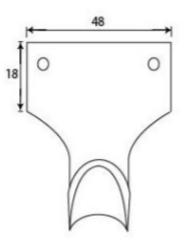
• Fixing plate: 48mm x 18mm
