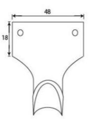
• Fixing plate: 48mm x 18mm
