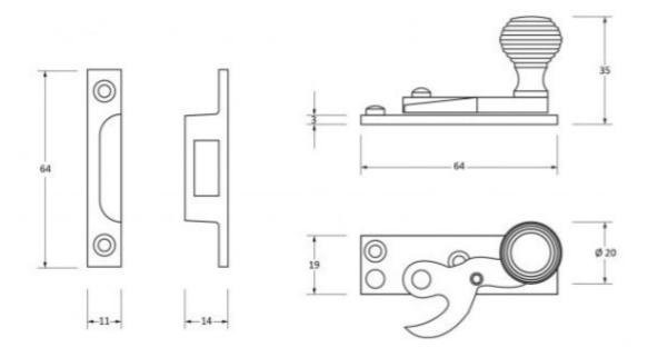
• Fixing plate: 64mm x 19mm
